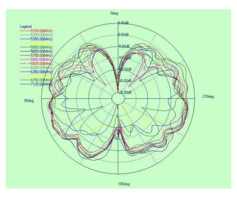
2D Radiation Pattern 5150~7125 MHz XY Plane
