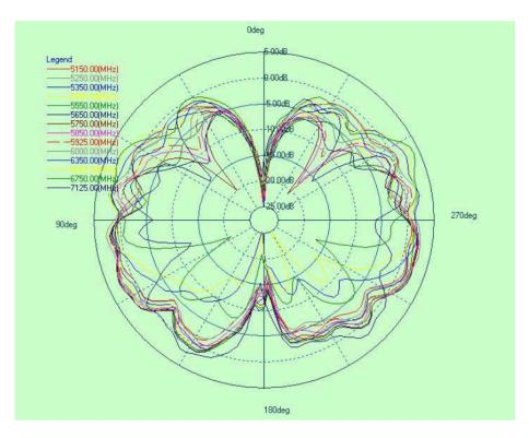
2D Radiation Pattern 5150~7125 MHz XY Plane
